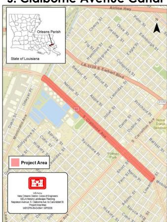
S. Claiborne Phase 1 - constructing approximately 2,600 linear feet of concrete canal under the inside west-bound lane of S. Claiborne Ave. from Monticello Ave. to Leonidas St.
