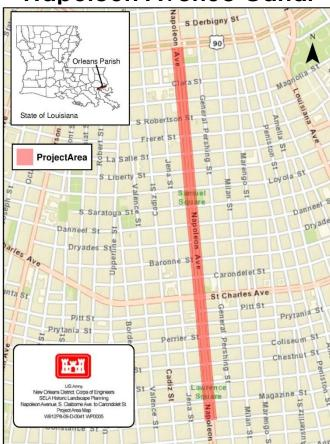
Napoleon Phase 2 - constructing approximately 4,100 linear feet of concrete canal under the neutral ground along Napoleon Ave... from S. Claiborne Ave. to Carondelet St.
