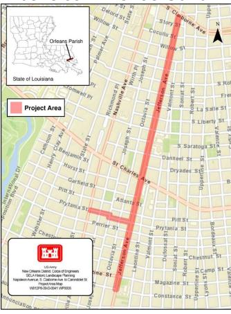
**Jefferson Phase 1** - constructing approximately 4.300 linear feet of concrete canal under the neutral ground along Jefferson Ave.. from S. Claiborne Ave. to Dryades Št.
